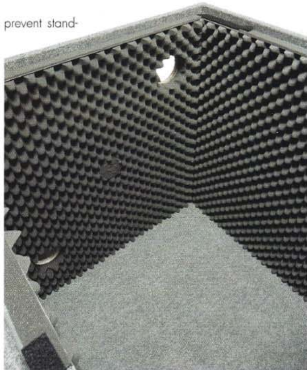
"standing waves" bouncing off of parallel reflective surfaces like floors and ceilings.
