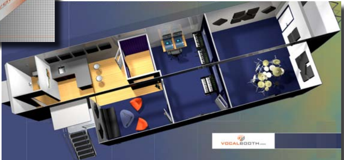
Below: This 54' VB Mobile Studio™ includes (from front to back): rest room, mini bar, lounge, VocalBooth™, control room, & performance space
